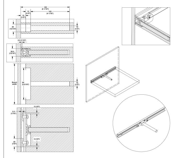
Proper routing for the shelf support and rail on rear edge of the panel will serve as an anti-tip feature when shelf is mounted. Applying a small amount of silicone adhesive will help secure the shelf support to the rail and panel.
